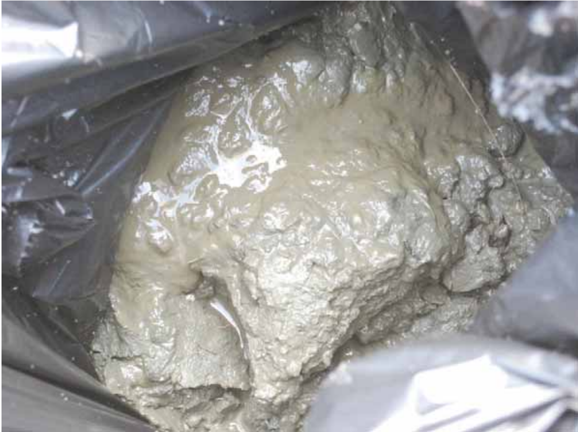
Figure 20: A sample of mud collected with the box corer, as it sits within the sediment receiver box shortly after recovery. The photo is included here to give readers an idea of sediment disruption when using this sampling technique.
