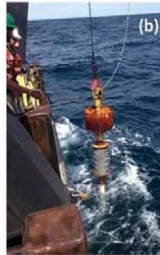
Figure 21: A schematic diagram of the gravity corer (a). Gravity core during use (b). Most of the elements of the corer used on this cruise are shown accurately in (a) except our apparatus used PVC pipe instead of a core barrel. The corer cutter [nose cone in (a)] and the core catcher were both affixed to the end of the PVC pipe. The corer valve, which allows water to flow out of the top as the core is penetrating the sediment, was built into the coupling shown in (a).
