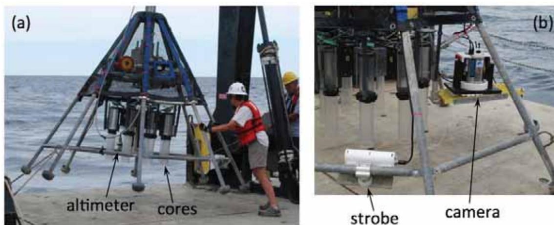
Figure 23: (a) Ellen Roosen (WHOI) and Chuck Dill (Alpine) deploying the MC-800 during the cruise. Also visible is the altimeter and the cores. (b) Alternative view showing the location of the bottom-imaging camera and the strobe. The strobe is also partially visible in (a) but the camera is mostly obscured in (a).
