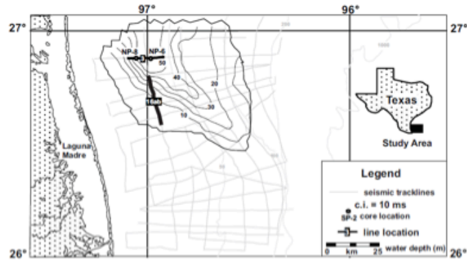
FIG. 17.—Isochron map of seismic unit Tst 4, which is interpreted as a hemipelagic mud blanket. Seismic lines 16ab (Fig. 17) and 3 (Fig. 18) are used to illustrate the seismic character of this unit.
