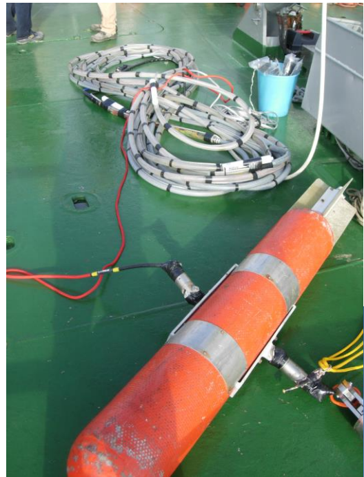
VLA (SLIVAI) : Reference array 32 elements 46.5 m long Spacing: 1.5 m
