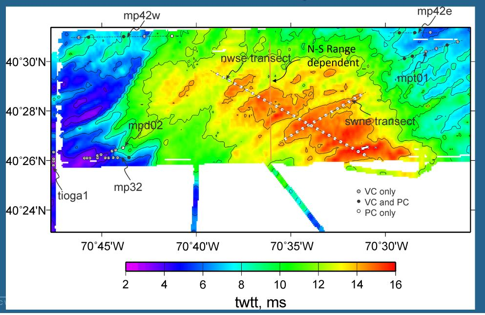
Mud layer thickness and comparison with chirp sonar survey results
